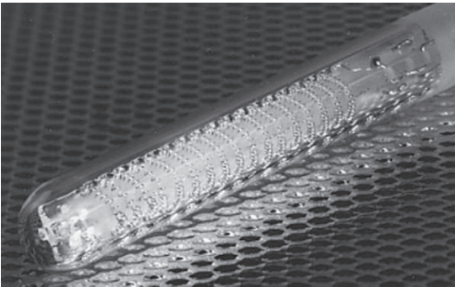
Figure 3.23 Typical measuring coil of a standard resistance thermometer for temperatures up to 1200°F
