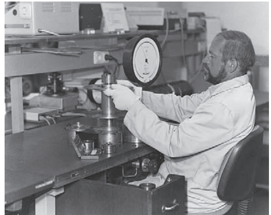
Figure 3.19 Calibrating a precision dial gauge with deadweight tester.
